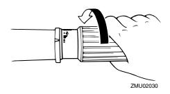
After the engine is at idle speed in gear move the gear shift lever firmly and crisply into the neutral position.
